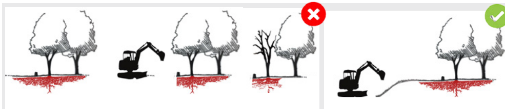
Fig.14 Standoff distance to prevent damage on the tree roots during works (© M.Profit, CLL)
